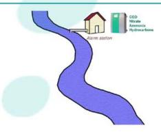
The concentration of ammonia in river water is an important parameter for drinking water treatment plants. Stability, reliability and low maintenance are the major concerns for these applications that only UV spectroscopy method can achieve.
